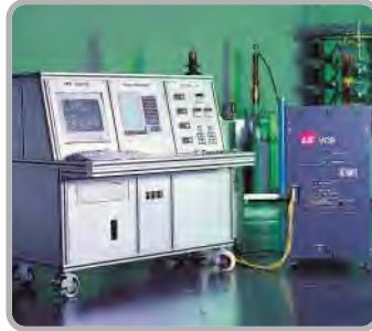
Characteristics Test / VCB Characteristics Test
